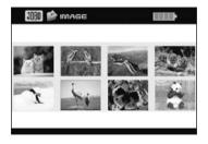
When you have selected a folder, press  $\square$  button for thumbnail view. Then 8 pictures are displayed on the screen. You can move through the whole folder by using the buttons:  $\blacktriangleright$ ,  $\blacktriangleleft$ ,  $\bigstar$  and  $\blacktriangledown$ . To start the slideshow press  $\square$  button again and the slideshow will start automatically. The pictures change automatically as well. To get back to the "Thumbnail view" just press again  $\square$  button.
